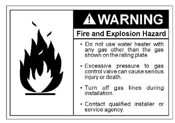
Make sure the gas supplied is the same type listed on the model rating plate. The inlet gas pressure must not exceed 14 inch water column (3.5kPa) for natural and propane gas (L.P.) gas. The minimum inlet gas pressure listed on the rating plate is for the purpose of input adjustment. If the gas control valve is subjected to pressures exceeding 1/2 pound per square inch (3.5kPa), the damage to the gas control valve could result in a fire or explosion from leaking gas.
